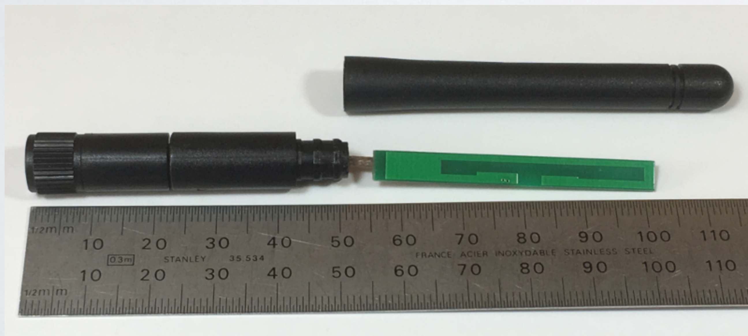
Antenna A: PCB antenna Not well tuned.
