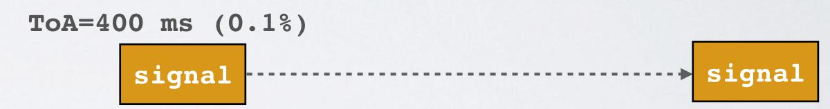
After 400ms of transmission time wait 999x400 = 399600 ms = 399.6 s (99.9%) for the next transmission.
