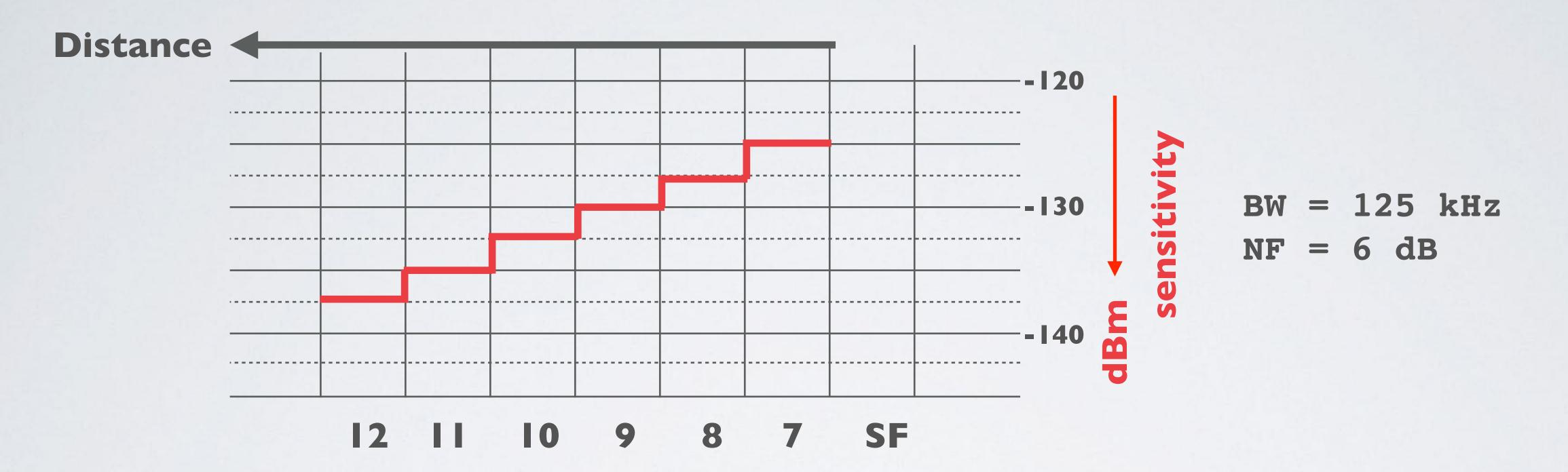
• If the distance between end node and gateway increases the signal gets weaker and therefore an increase spreading factor is needed for a lower receiver sensitivity to be able to demodulate the received signal. The Spreading Factor ranges from 7 when close to a gateway to 12 when far away from a gateway.
