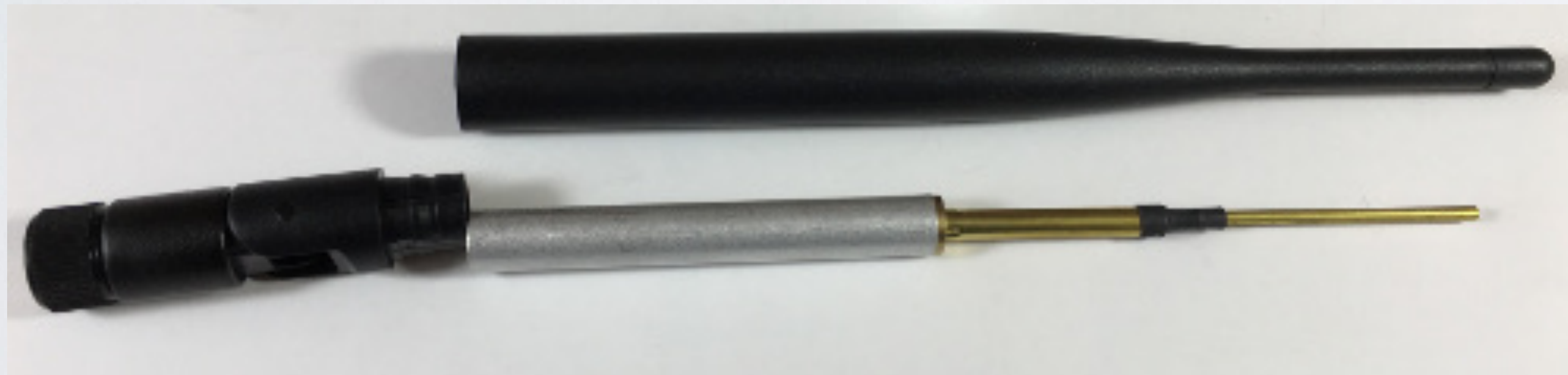
Antenna B: Sleeve dipole antenna
