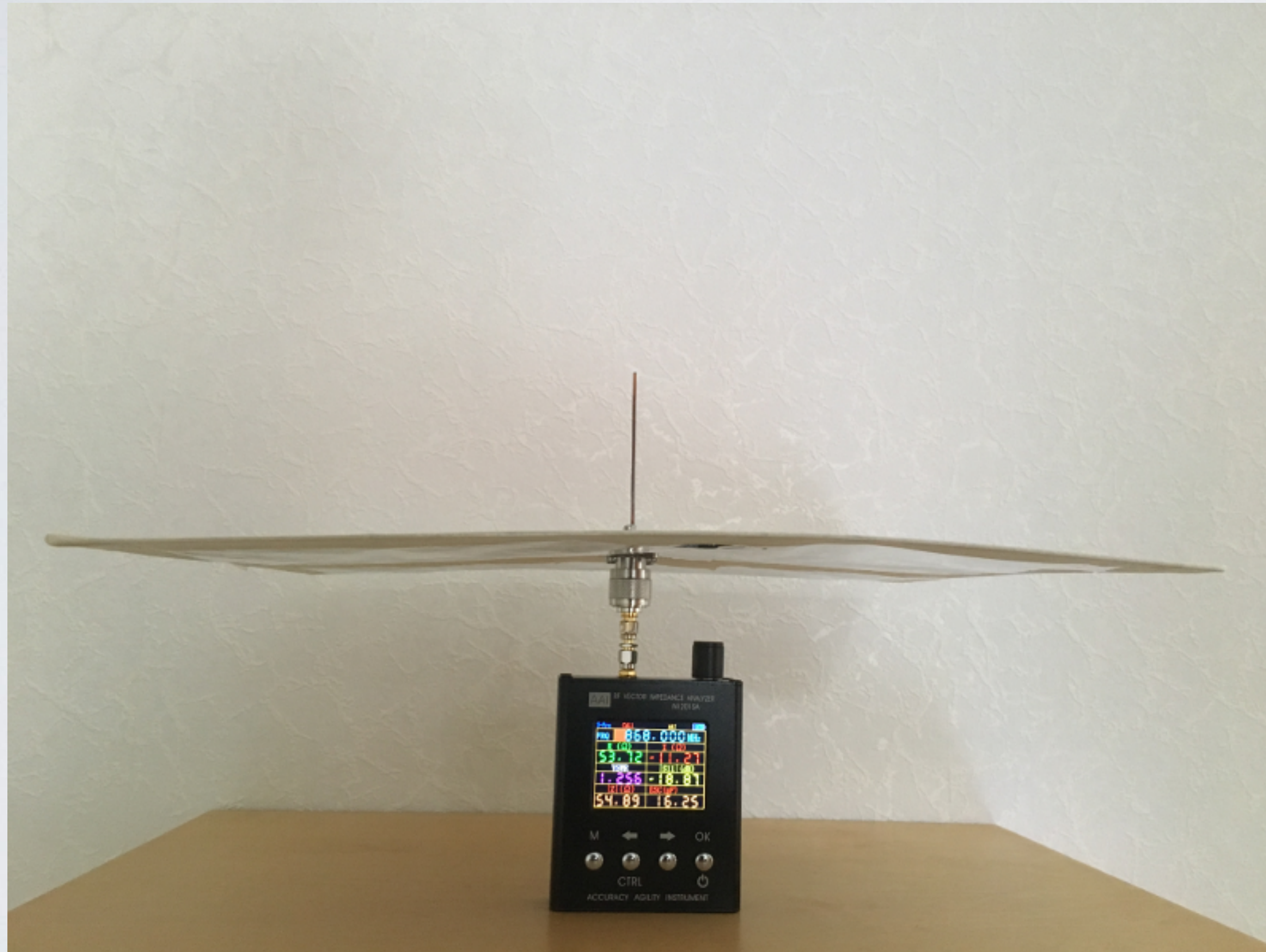
Measuring antenna parameters
