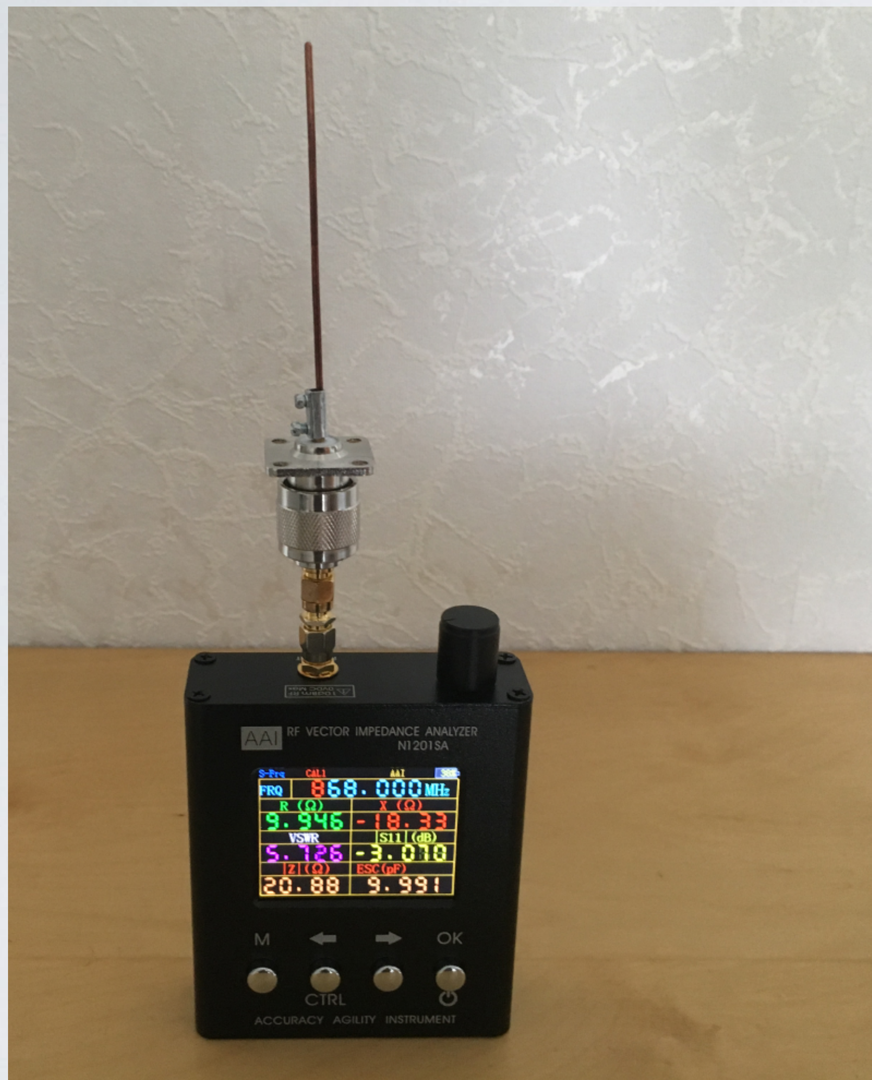
Measuring antenna parameters
