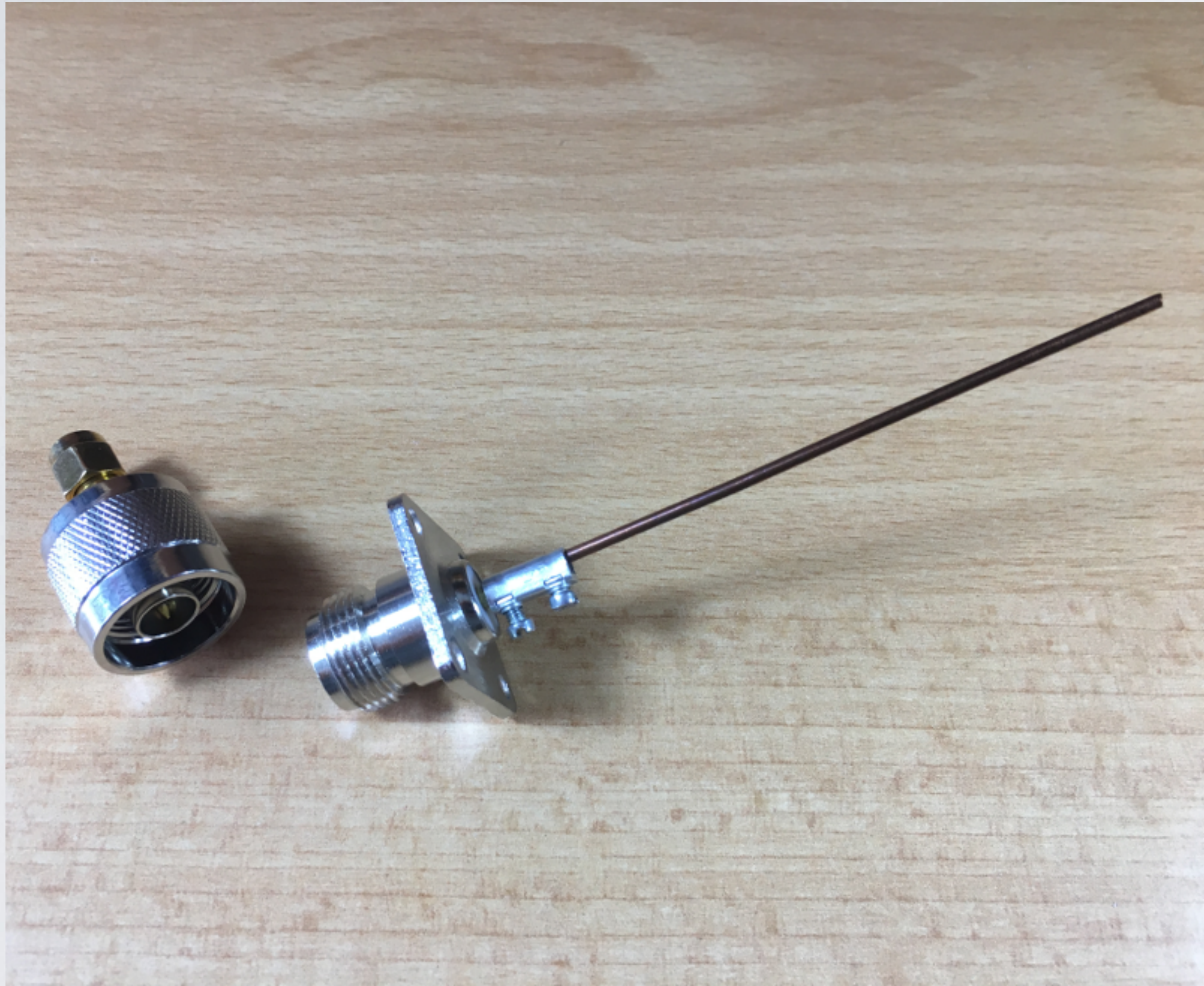
Assemble monopole antenna
