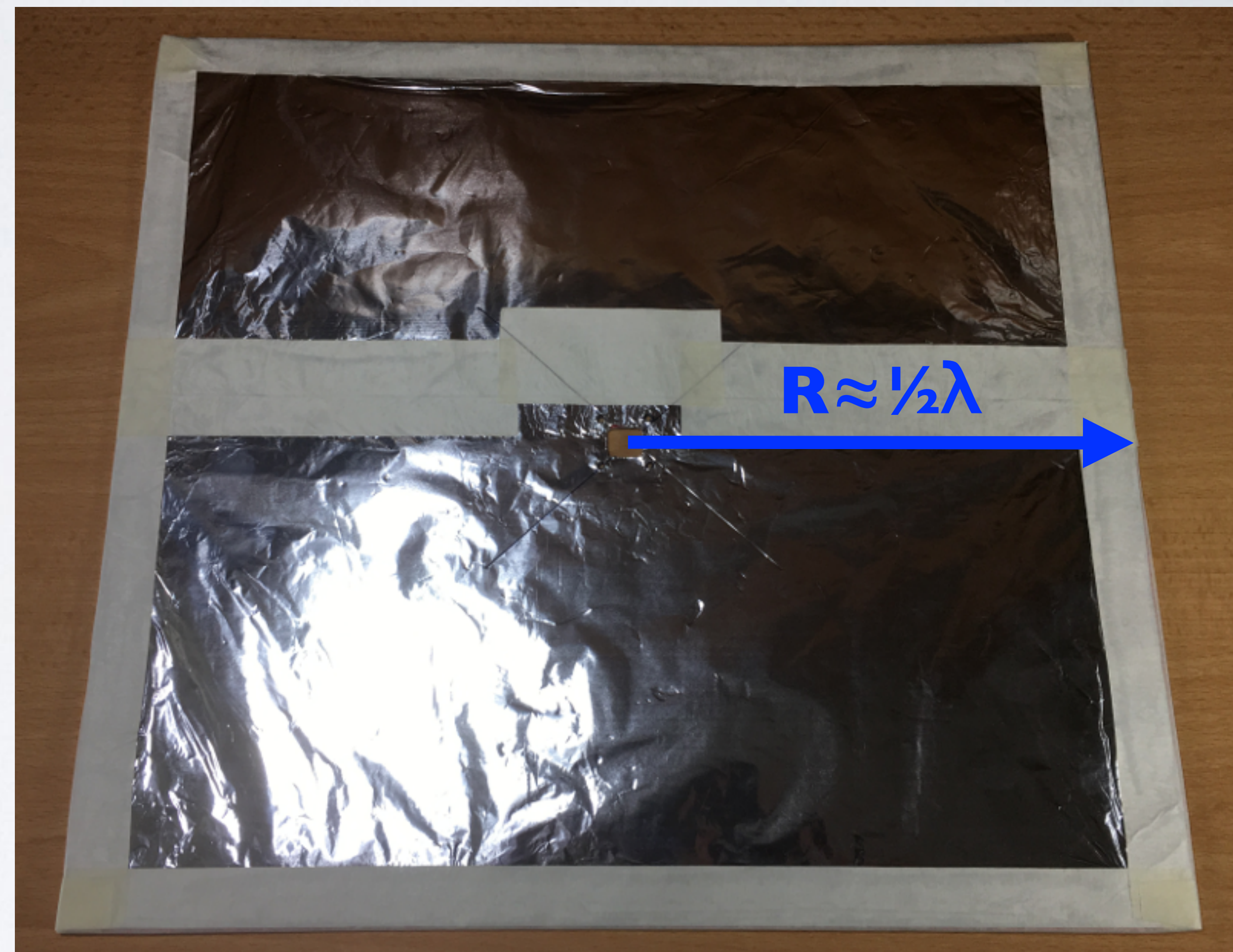
Ground plane B size 335 mm x 369 mm
