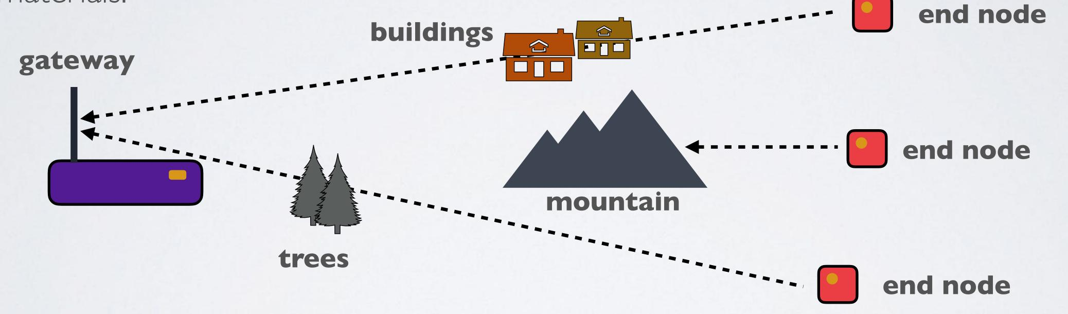
Buildings are made of more conductive materials which weakens the signal more compared to trees. A mountain blocks the signal completely.
