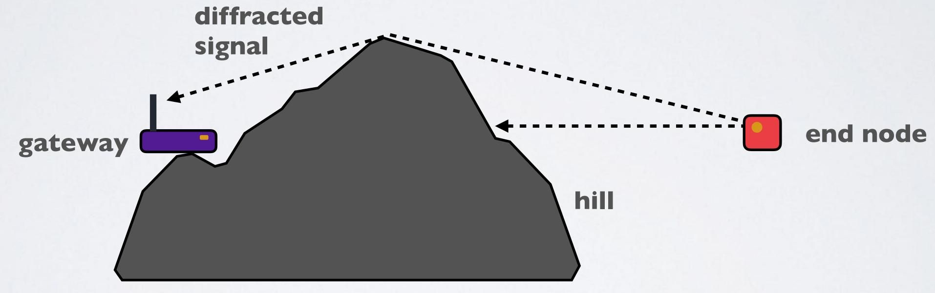
Gateway receives the diffracted signal but not the direct signal
