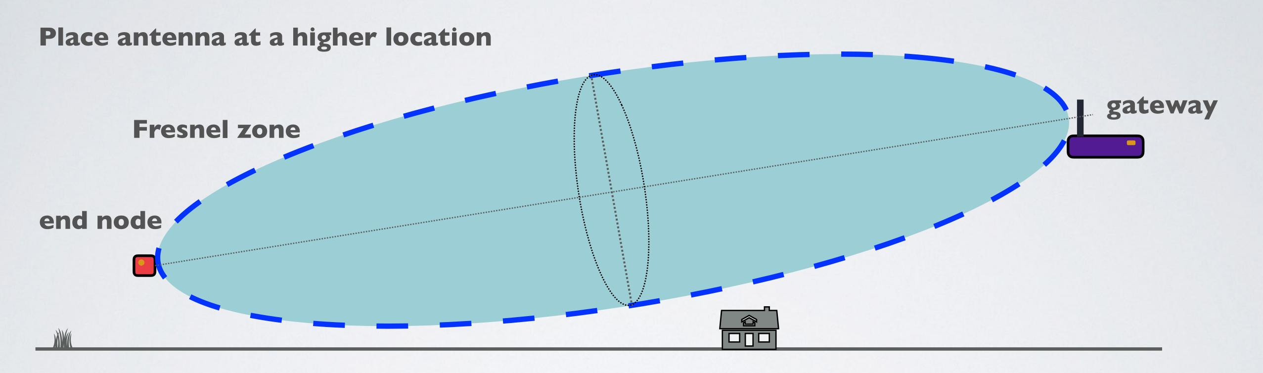
End node sends signal to gateway without any interference No obstacles in the Fresnel zone
