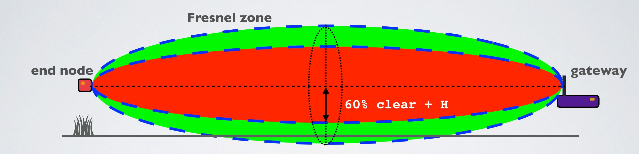
Example: f = 868 MHz = 0.868 GHz H is the earth curvature allowance.
