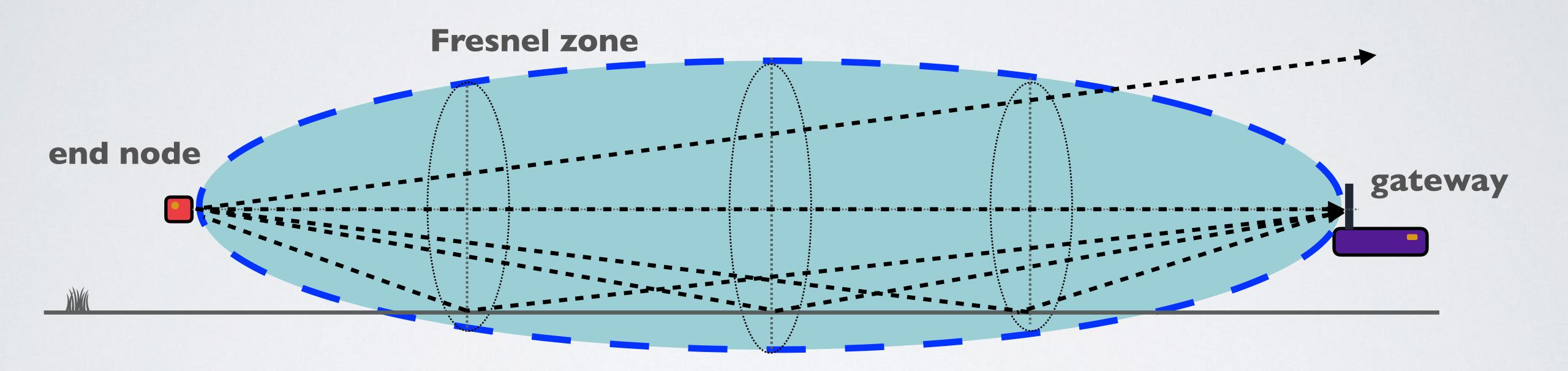
Ground is inside the Fresnel zone Reflected signals interfere with the direct signal
